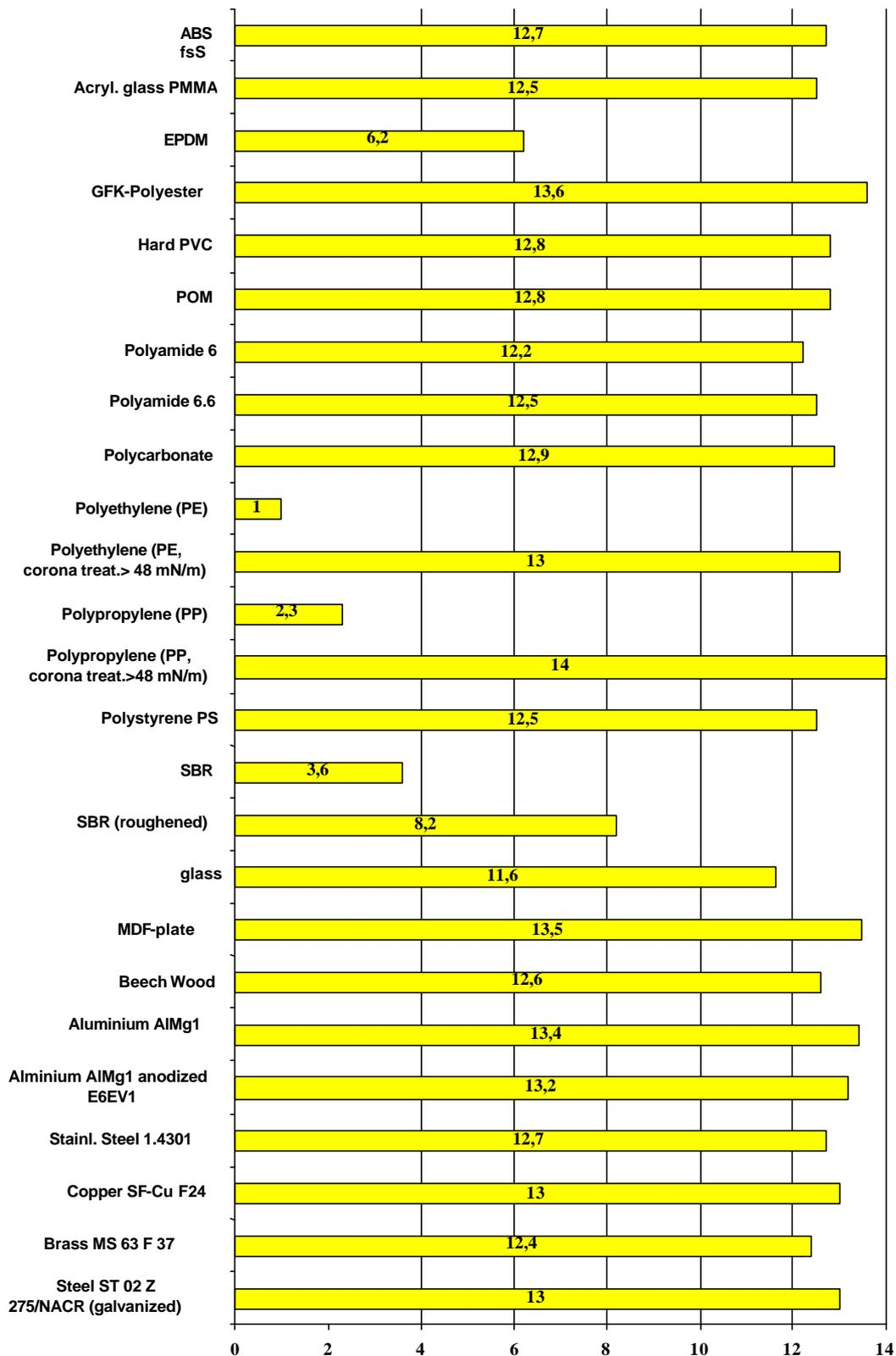
Peel strength measured as per PSTC 1 with peel tester type L 500 of Lloyd Instruments, load cell 100 N, class 1, DIN EN ISO 7500-1 for tension and pressure, 180°C peel test, printed with a 350 µm steel mesh onto 50 µm PET film, measured after 72 hours storage at ambient temperature (as per DIN 50014-20/65-1), in N/cm. Peel speed 300 mm/min. Adhering with hand roller (as per PSCT standard, roll weight 10 pounds, 5 x in each direction). Adhering area: 2,5 x 10 cm.
